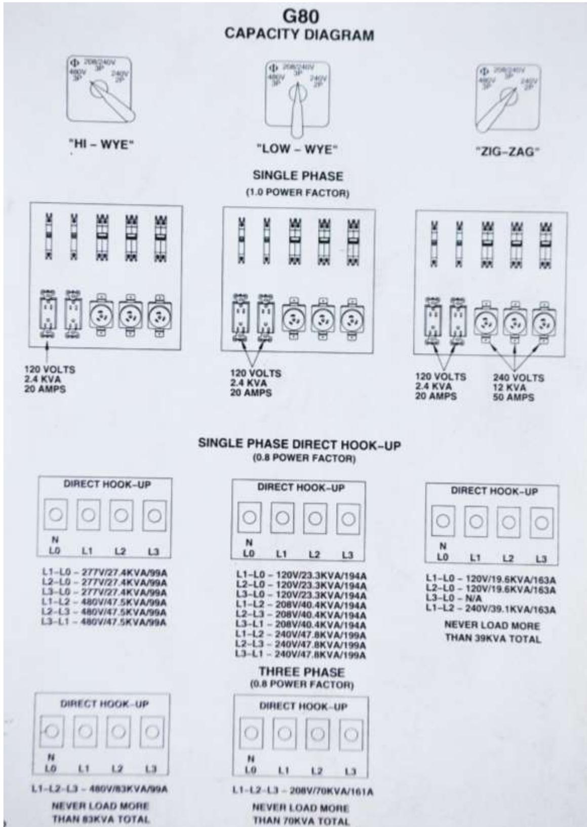
**Danger:** Never change the Voltage Selector Switch when the Engine is Running!
